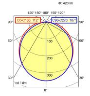
light sourceLEDwork equipmentwithoutconnected load22-26 V, DCpower consumptionenv. 16 Wluminous fluxapprox. 420 lmluminous efficiencyapprox. 26 lm/W
